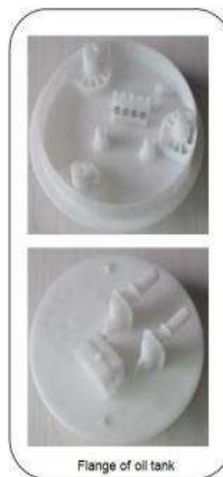
Flange of oil tank
